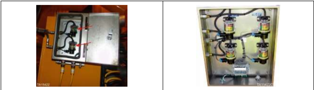
Some machines have two and some have four restriction gauges, depending on engine manufacturer
