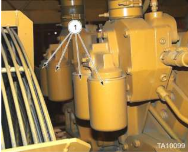
1) Coolant Conditioning Filters (Mounted at top – front of engine - Cummins engine shown)
