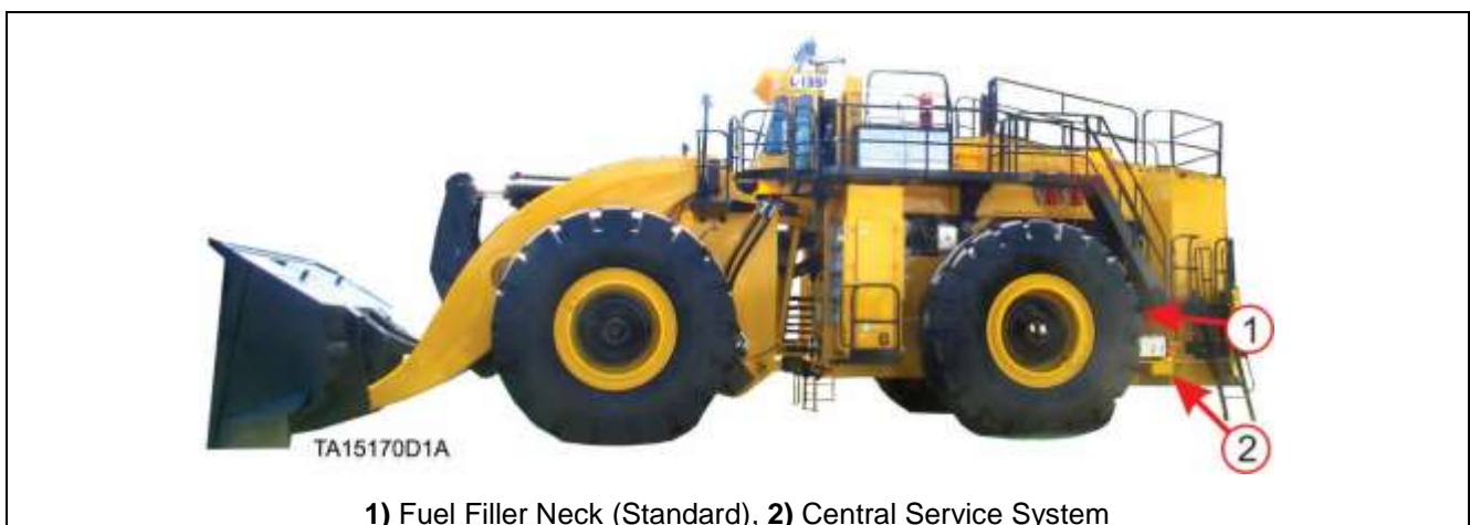
Figure 2. Typical fuel filler location
